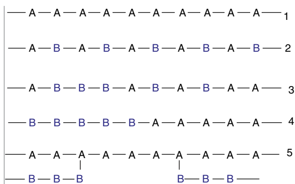
Fig. 4.6 Structures of homopolymers and copolymers composed monomers A and/or B. (1 linear homopolymer, 2 alternating copolymer, 3 random copolymer, 4 block copolymer, 5 graft copolymers) ( https://en.wikipedia.org/wiki/Copolymer#/media/File:Copolymers.svg )
