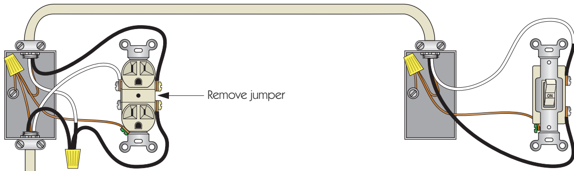
SPLIT-SWITCHED RECEPTACLE (top receptacle switched)
