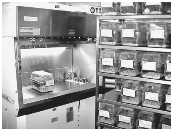
Figure 8.27 A rack with static microisolation cages adjacent to a Type II A biosafety cabinet with a microisolation cage inside the cabinet. The combination of the microisolation cage and cabinet makes up what is known as a “microisolation cage system.” The microisolation cages are only opened inside the cabinet, including for cage changes or research procedures.
