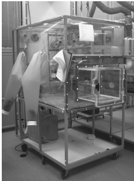
Figure 8.30 Flexible film isolator. The isolator in the photo has a large square entrance port, which is easier to load than the more common circular ports.
