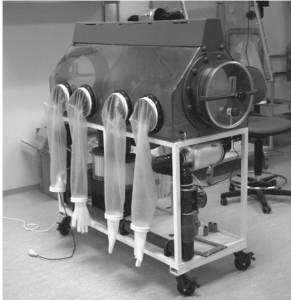
Figure 8.31 A rigid stainless steel isolator that was specially adapted to perform hysterectomies for rederivation of animals. The isolator is divided into two parts, one in which the hysterectomy is performed and one where the pups are resuscitated. The two parts are separated with a dip tank containing a disinfectant.
