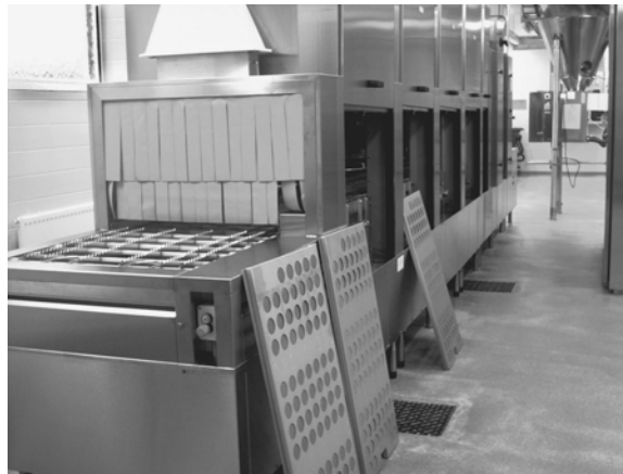
Figure 8.22 A continuous belt tunnel washer designed for use with robots that load and unload cages from the belt. It has two features that are required to accommodate robots: (1) it is an indexing tunnel washer that stops periodically for loading and unloading the belt, and (2) it has exceptionally long load and unload extensions that can accommodate several rows of cages as opposed to the more typical extensions that may hold only one row of cages. The dividing wall for separating the clean and soiled sides of the cage sanitation area is not yet in place.
