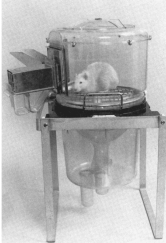
Figure 15.39 Sampling urine and feces from a rat using a metabolism cage. (Techniplast Gazzada S.A.R.L., Italy.)
