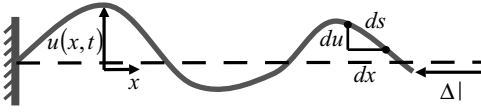
Fig. 8-3. From one fixed end, a filament tends to wander in a way that can be characterized by u(x) , the transverse displacement from an initial straight line (dashed). If the arc length of the filament is unchanged, then the transverse thermal fluctuations result in a contraction of the end-to-end distance, which is denoted by \Delta\ell . In fact, this contraction is actually distributed about a thermal average value \langle\Delta\ell\rangle . The mean-square (longitudinal) fluctuations about this average are denoted by \langle\delta\ell^2\rangle , while the mean-square lateral fluctuations (that is, with respect to the dashed line) are denoted by \langle u^2\rangle .
