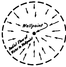
Figure 12-4 Flow of Water From Aquifer to Well Point.
