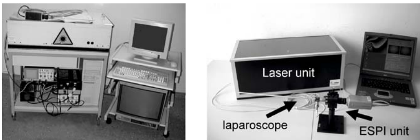
Fig. 9.4. ( Left ) Mobile endoscope ESPI system based on an analog CCD camera and an image processing system with frame grabber interface. ( Right ) Modular endoscope ESPI system with IEEE1394 (“FireWire”) technology consisting of a laser unit, a speckle interferometric module, and a notebook-computer for image processing
