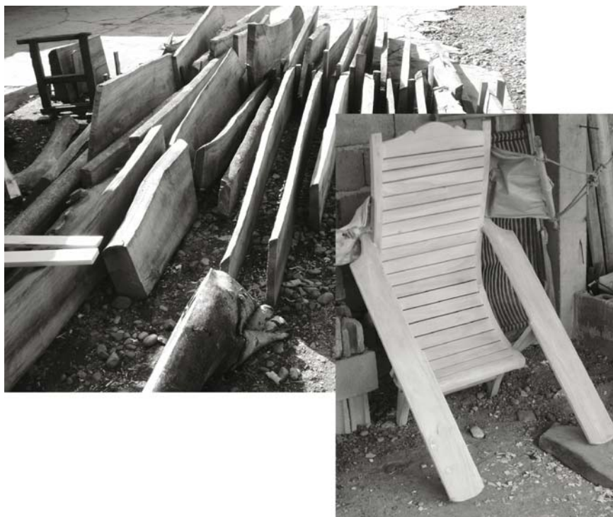
Photo 8.1 Gmelina arborea planks drying and finished product on a smallholder's compound in the Philippines (©DJ Snelder)
