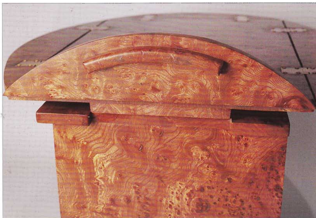
BELOW: Sides of tray showing handle and feet which act as locators
