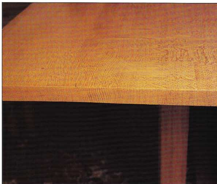
ABOVE: Quarter-sawn oak end-grain table top — right
