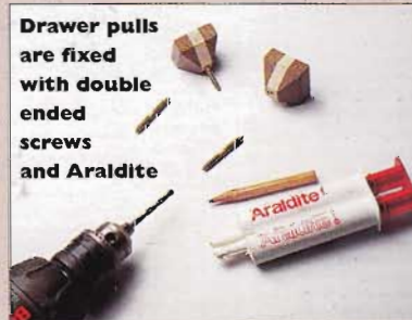
Construction of drawer pulls
