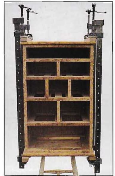
ABOVE LEFT AND RIGHT: Cramping up has to be done in sequence
