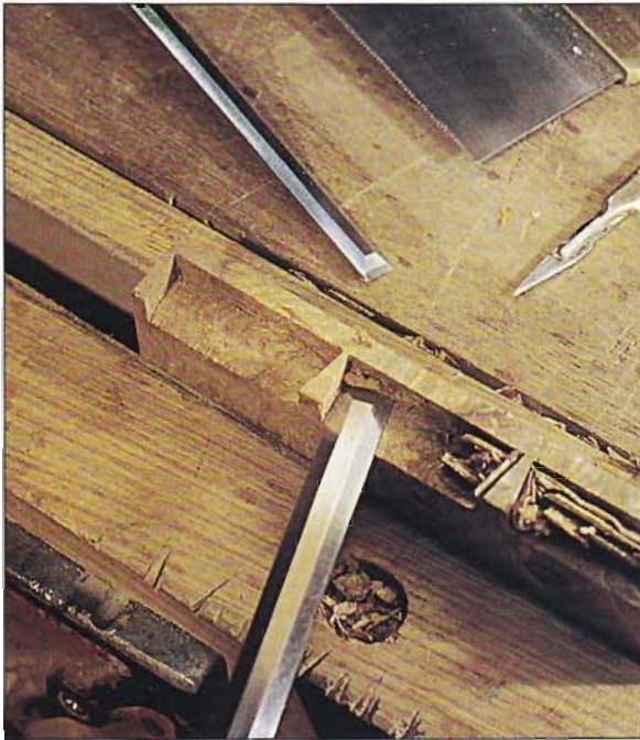
ABOVE: Sharp tools and care are needed to avoid chipping the burr
