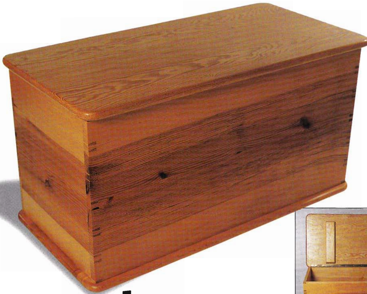
LEFT: Photo 1 Pine blanket box showing grain direction around sides
