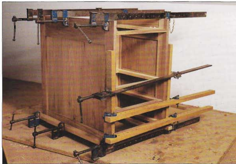
LEFT: Cramping the pedestal
