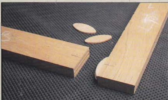
Double biscuit joints have proved to be more than adequate as an alternative to loose tenons
