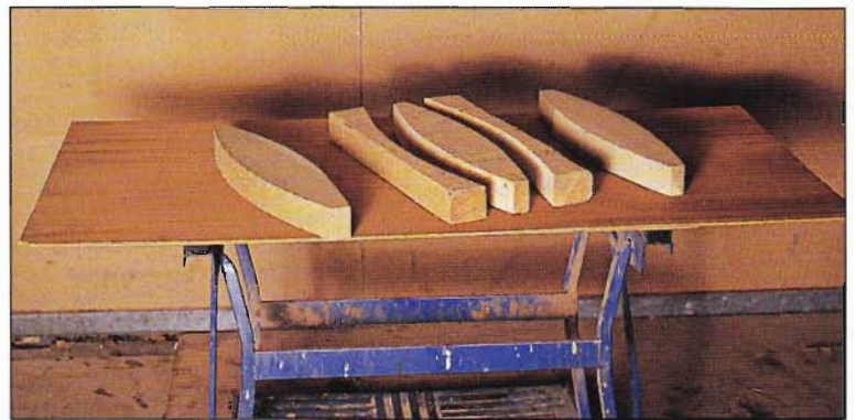
ABOVE: A simple former for producing the steam-bent back rails
