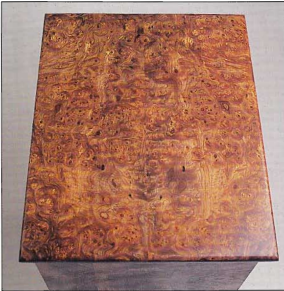
ABOVE: Careful matching of boards for the top and drawer fronts
