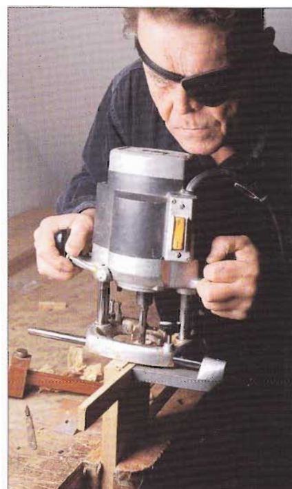
Routing waste from dovetails
