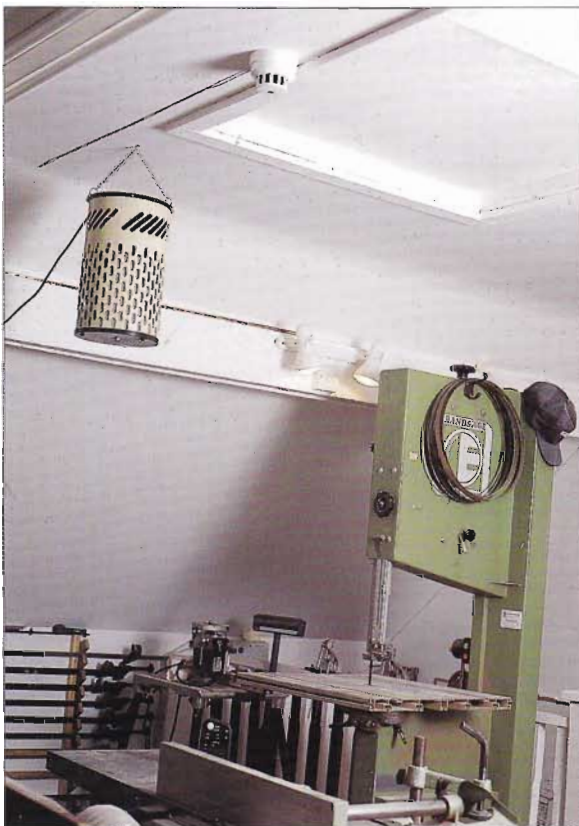
BELOW! Microclene air filter mops up ambient dust
