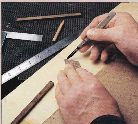
ABOVE: Marking inlay with a scalpel
