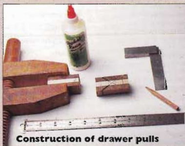
Drawer pulls are fixed with double ended screws and Araldite
