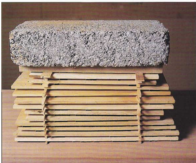
ABOVE: Drawer casings in stick with a weight on top
