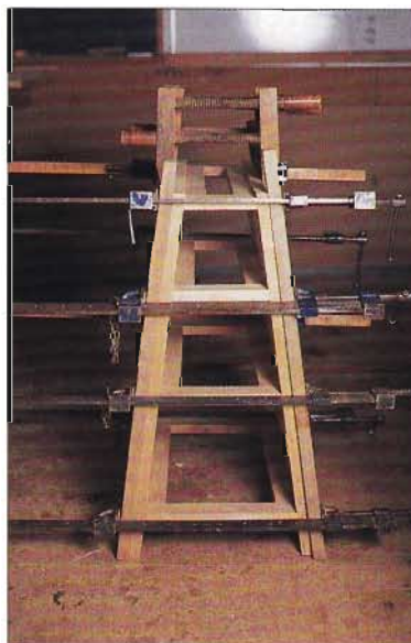
LEFT: Another tapered carcass being cramped up showing cawls to ensure even pressure on all joints
