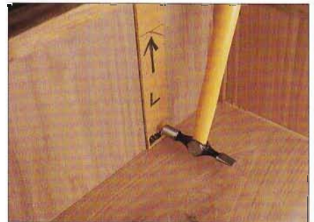
BELOW: Using hardboard jig for fixing the panel pins in the backs
