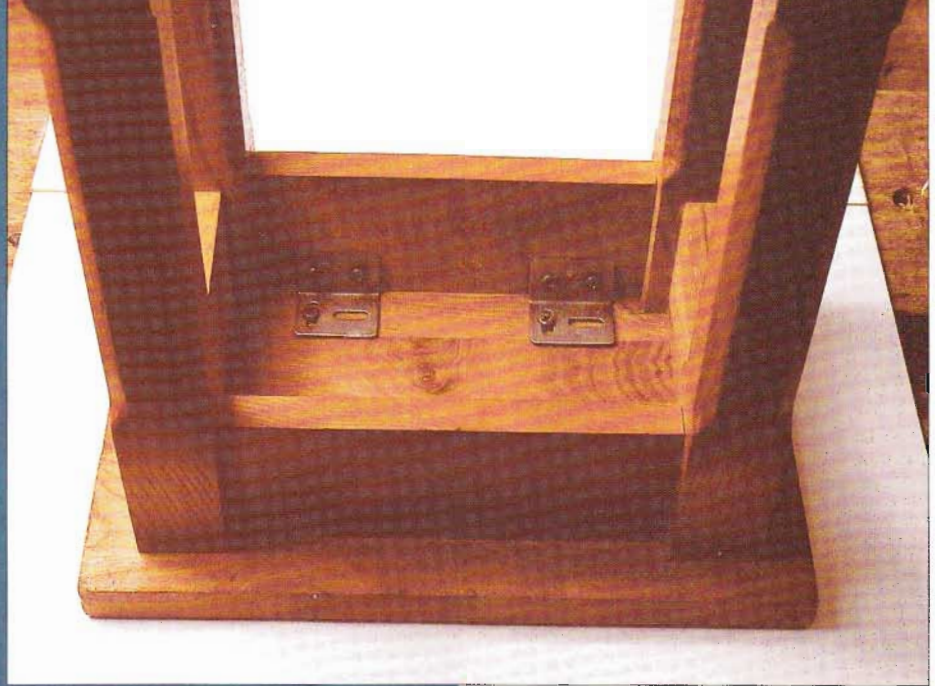
The expansion plates on the smallest of the three tables
