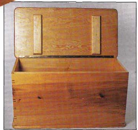
BELOW: Photo 2 Lid open, showing braces
