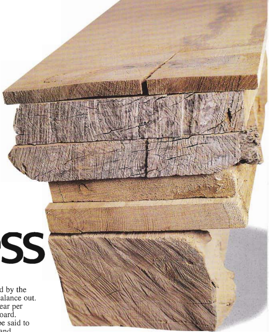
ABOVE: End-grain, split and unpainted
