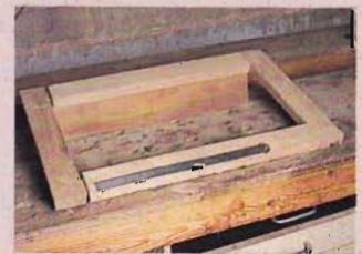
ABOVE: Photo 5 Drawer frame showing expansion gap
