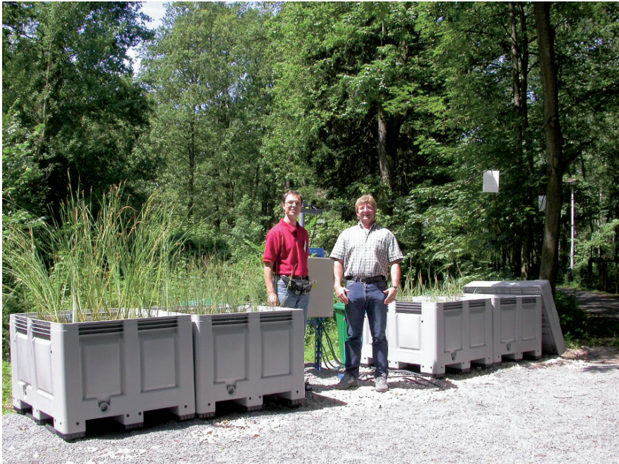
Figure 6. Pilot constructed wetland – each container volume is 1 m 3 .
