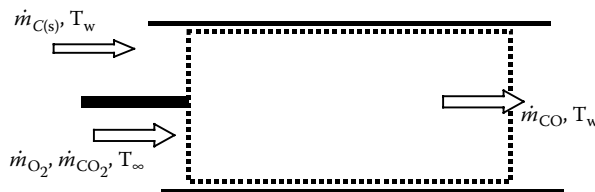
Figure P.9.14 T_w of gas leaving the vector is the same as the adiabatic flame temperature. Figure for Problem 9.14.
