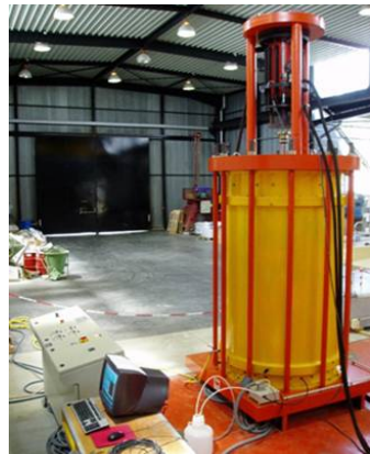
FIG. 1. First configuration (right) and second configuration (left) of the large triaxial cell.
