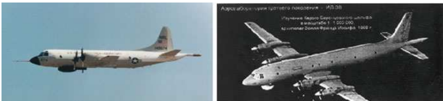
Fig. 3.1 Left: Orion P-3 aircraft used in the US NRL airborne gravity program; right: IL-76 geophysical laboratory used in the PMGRE Russian polar airborne gravity program. Photos courtesy J. Brozena (NRL) and M. Sorokin (PMGRE)
