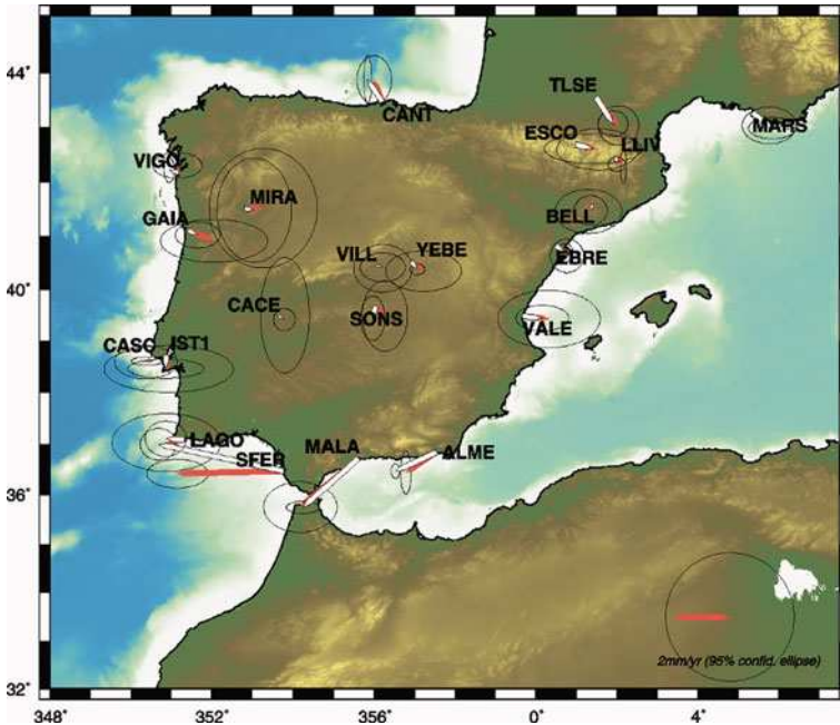
Fig. 5.10 Velocity field (w.r.t. Nubia) before ( grey ) and after filter ( white ) (Bastos et al. 2006)
