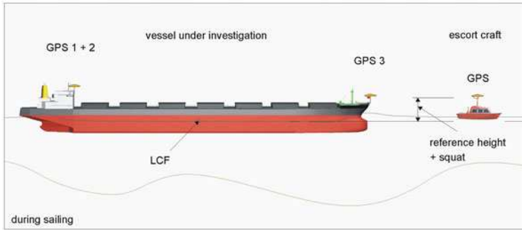
Fig. 8.18 Principle of SHIPS method
