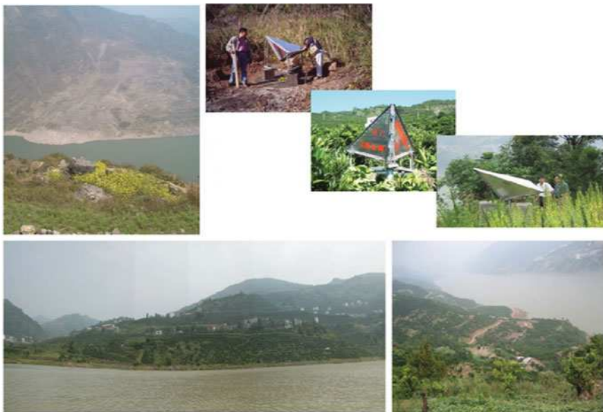
Fig. 11.25 Photos of the landslides and reflector corners
