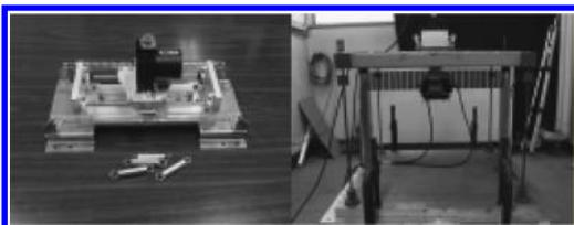
Figure 1. Variable Pendulum Sensor and Experimental structural model.
