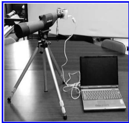
Photo 1. Displacement measuring system.
