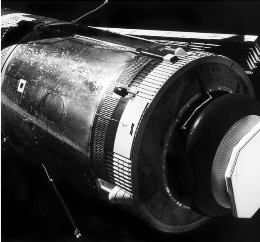
17. The exterior of the Orbital Workshop, stripped of its heat shield, began to bake in the solar radiation.
