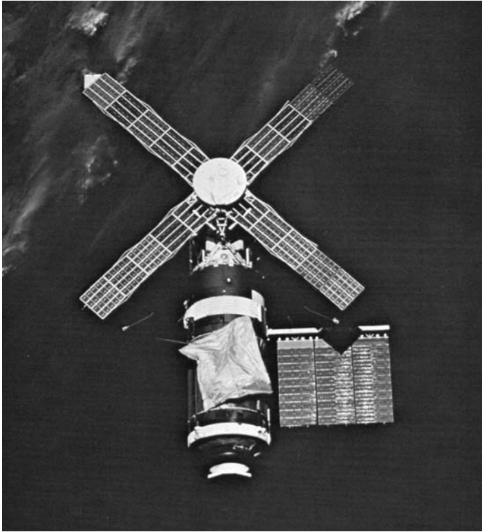
25. The sun-shield parasol, as deployed by the first crew of Skylab.
