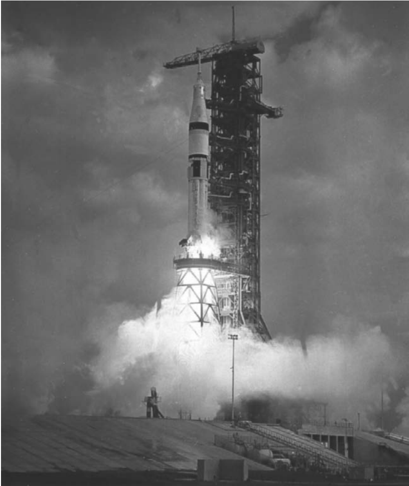
23. The “milkstool” used to raise the Saturn IB boosters for launch on the Saturn v–fitted launch pad is visible in this photo of the SL-2 launch.
