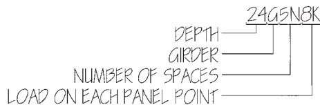
FIGURE 7-6 Joist Girder Designation
