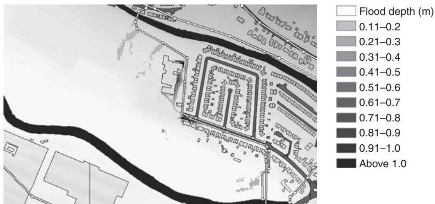
(a) start of flooding – water surcharging from sewer manholes
