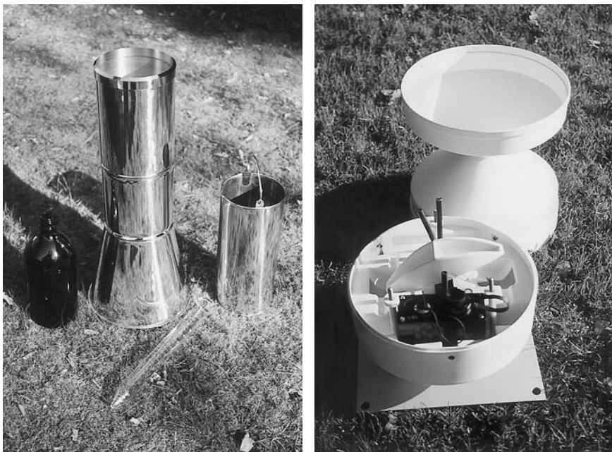
Fig. 5.1 Rain gauges: (a) standard; (b) tipping bucket (courtesy of Hydrokit, Poole)
