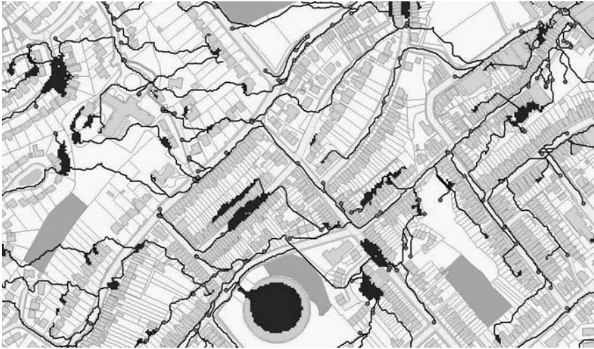
Fig. 20.6 Example of automatically generated network of surface flow pathways and ponds (courtesy of Professor Cedo Maksimović)
