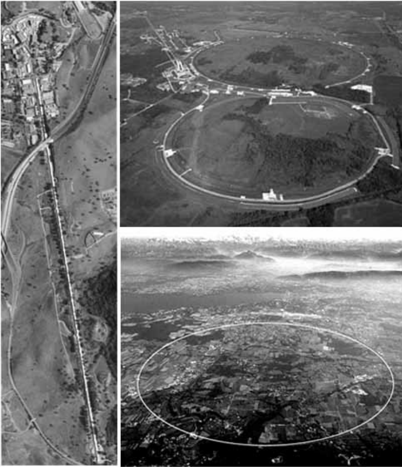
Fig. 15.2 Cathedrals of our time: large particle accelerators. Left: SLAC (Stanford Linear Accelerator) near San Francisco, a 3 km perpendicular bisector of the San Andreas fault, accelerates electrons to 50 GeV. Right top: booster and main ring of Tevatron collider at Fermilab near Chicago. It accelerates protons to 1 TeV. At one time, areas within the rings were planted with prairie grass kept trim by a herd of buffaloes. Right bottom: white circle marks position of underground accelerator ring, 8.5 km in diameter, of the Large Hadronic Collider (LHC) at CERN (Conseil Européen pour la Recherche Nucléaire), Geneva, Switzerland. When completed in 2007, it will accelerate protons to 7 TeV. The Jura mountain range looms at top of picture.
