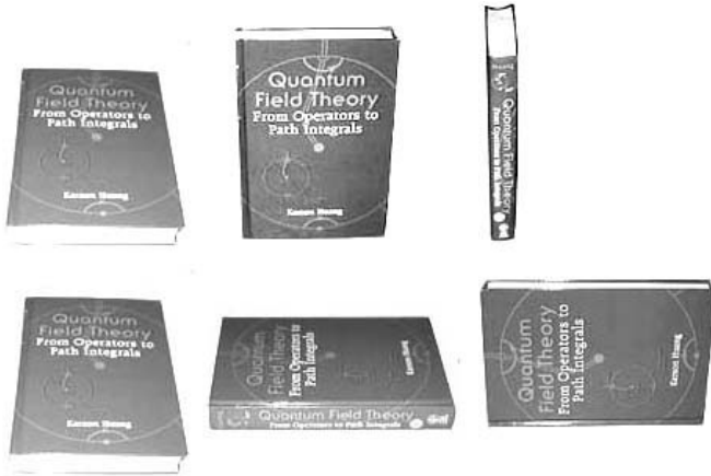
Fig. 8.1 Rotations do not commute: A book is rotated successively about a horizontal axis and a vertical axis, in different orders, with different results. Top row: 90^\circ about horizontal axis, then 90^\circ about vertical axis. Bottom row: same rotations in reversed order.
