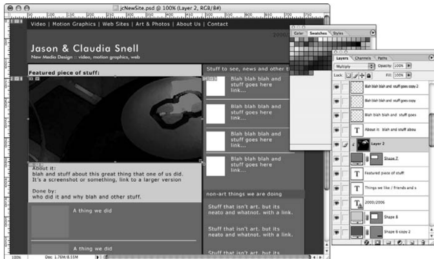
Figure 7-9: Slice only those areas that need to be graphics. Text and large areas of solid color are taken care of in the HTML.
