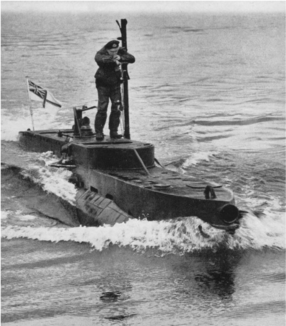
A British midget submarine on the surface. There is no conning tower and the officer taking bearings is strapped to the periscope stanchion to prevent him being swept overboard.
