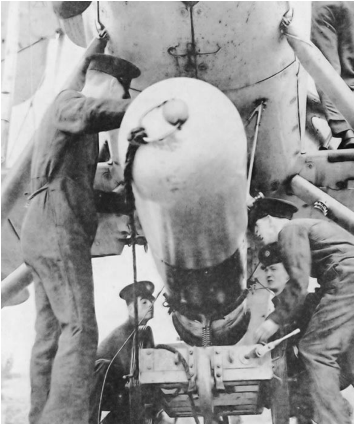
A torpedo is being fitted to the underside of a Swordfish aircraft by armourers and aircrew.
