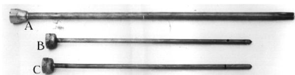
Figure 9.2 Injection nozzles: soil injector (top); cavity/ ventilator injector (middle); sill injector (bottom)
