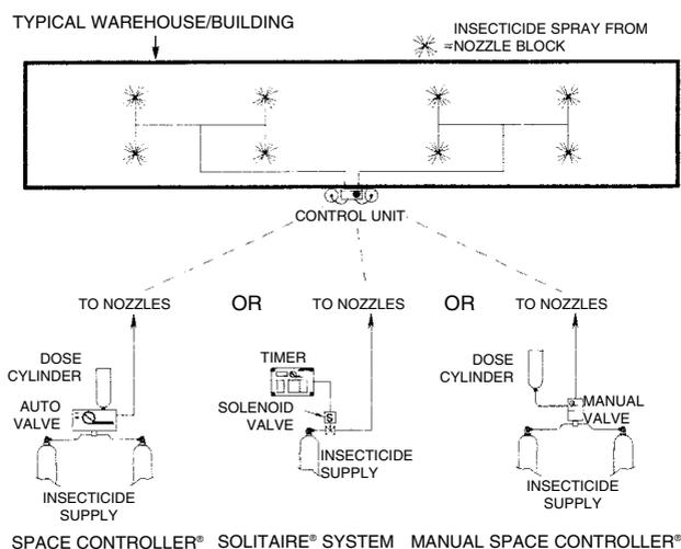
Figure 9.17 Diagrammatic representation of Envirosol® automatic dispensing systems
