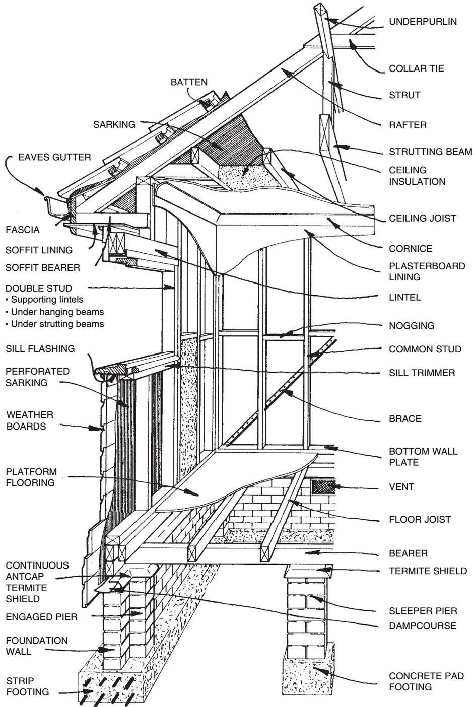
Figure 2 Timber framed construction
