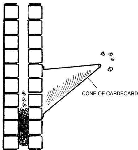
Figure 16.1 Cone device for removing honey bee activity from a cavity wall
