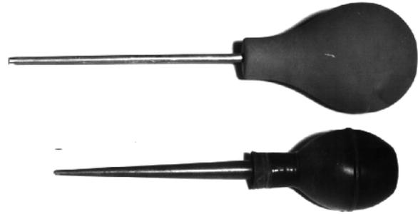
Figure 9.8 Hand-puffer type dusters: Cockroach duster (top); Termite duster (bottom)
