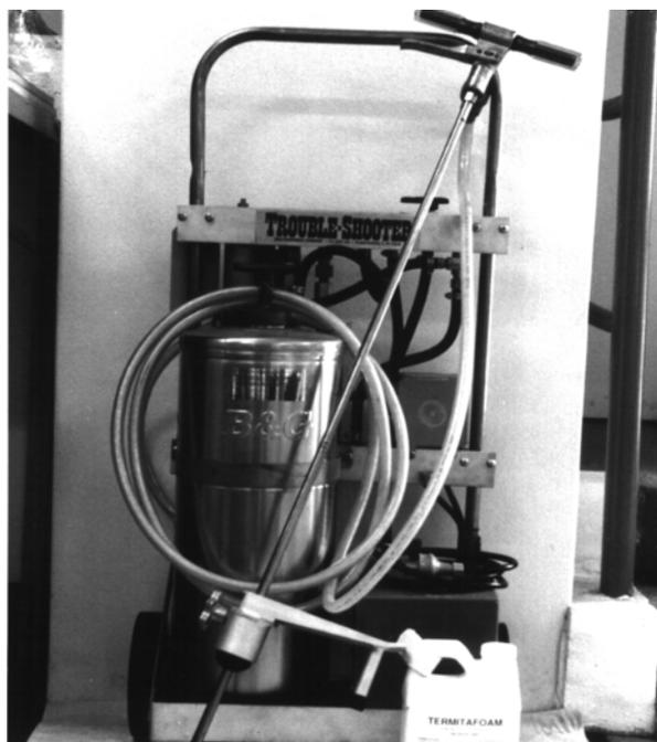
Figure 9.4 B+G Trouble-Shooter Portable Foaming Unit
