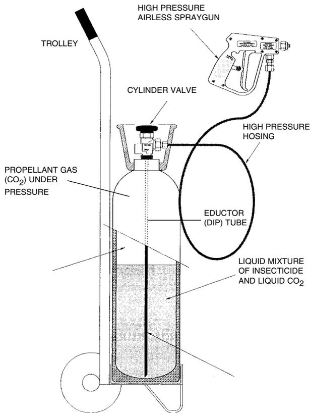
Figure 9.14 Section diagram of high-pressure aerosol system which utilises a liquid carbon dioxide propellant and solvent system
