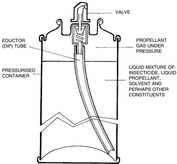
Figure 9.13 Section diagram of typical low-pressure aerosol container
