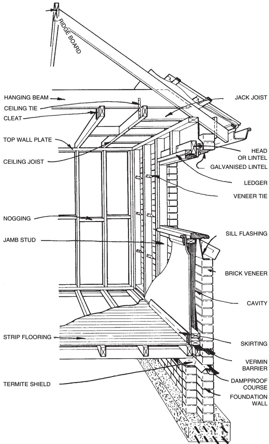
Figure 3 Brick veneer construction
