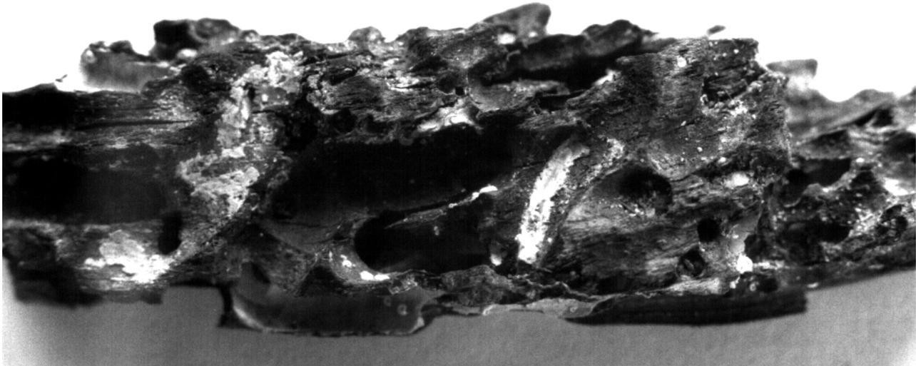
Figure 21.8 Mollusc marine borer damage. Note the holes lined with a calcareous material.
