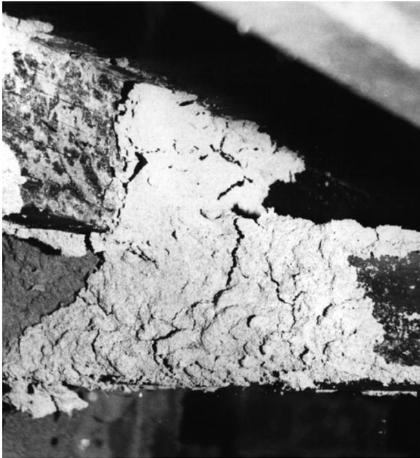
Figure 19.10 Packing and access galleries of *C. acinaciformis*
