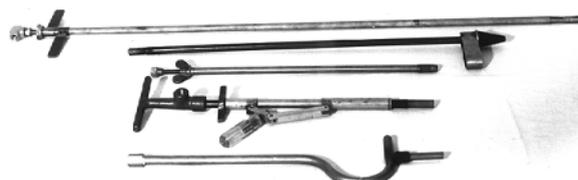
Figure 9.3 Various types of slab injectors
