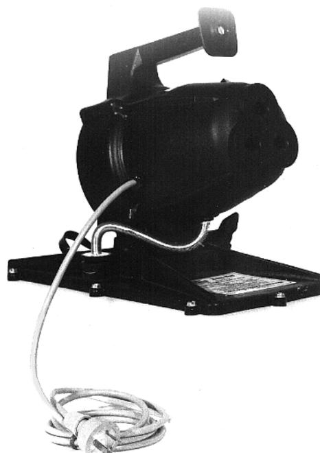
Figure 9.12 Cold aerosol generator: DC-3 Curtis Dyna-Fog, 240V
