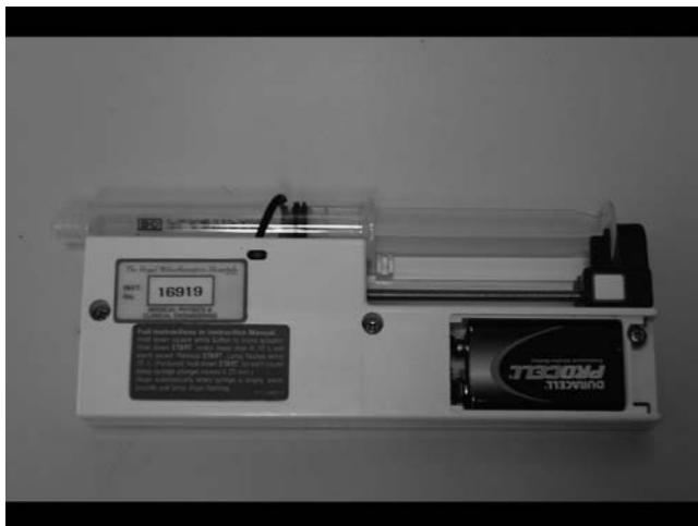
PHOTO 2.2. A battery-driven chemotherapy pump (courtesy of Mr Simon Glazebrook, New Cross Hospital Wolverhampton) (See Color plate 1)
