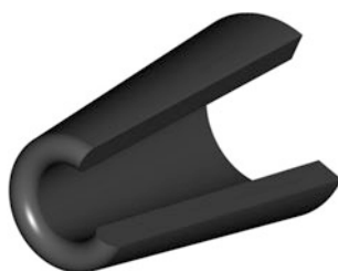
Fig. 7.19 A schematic of a micropipette tip. If the tip is formed in a fluid phase then the tip should have a hemispherical shape
