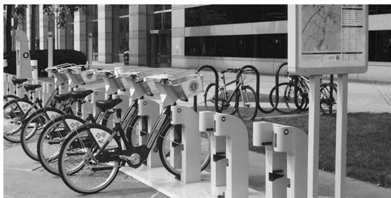
Figure 5.2 Charlotte B-cycle station which includes stalls for 20 bicycles, map of the city with other stations, and payment kiosk.
