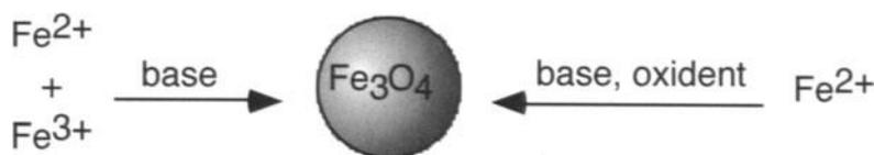
SCHEME 1.6. Aqueous preparative methods for the synthesis of iron oxide MNPs.
