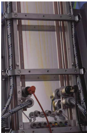
FIGURE 2 Performance test to check the functionality of the Pro Team FFE instrument. Red and the six yellow markers are separated according to their different pI values and mimic the actual separation of the proteins.
