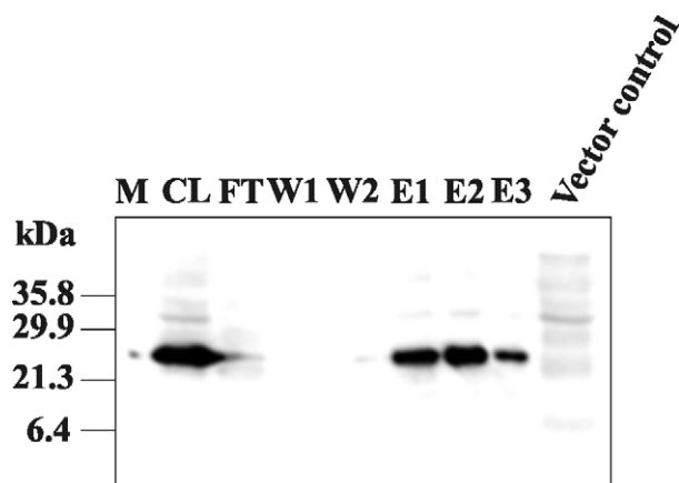
FIGURE 1 Expression and purification of the His 6 /StrepII-tagged human G-substrate protein (21 kDa) from S. cerevisiae as an example. Cleared cell lysate (CL) was prepared and expressed protein purified via Ni-NTA. A clone carrying an empty expression vector was used as the negative control (vector control). The proteins were separated by SDS-PAGE and detected by immunoblotting with StrepTactin HRP conjugate. M, prestained Bio-Rad broad range marker; FT, flow through from Ni-NTA column; W1, wash fraction 1; W2, wash fraction 2; E1-E3, eluates 1-3.
