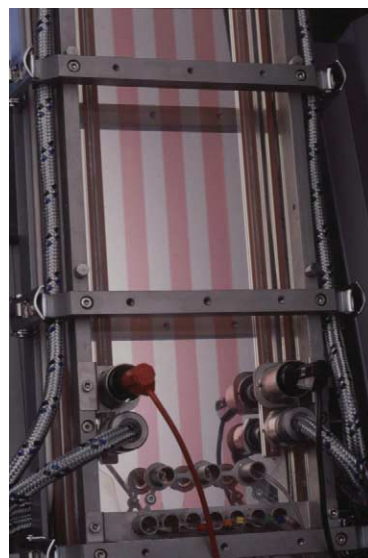
FIGURE 1 Stripe test to check the flow profile and the proper assembly of the Pro Team FFE instrument.
