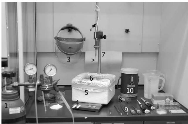
FIGURE 3 Working setup as typically used for freeze plunging. (1) caseous ethane bottle, (2) regulator valve with Tygon tubing and pipette tip, (3) full face shield, (4) filter paper strips, (5) polystyrene box for liquid nitrogen, (6) small container (sitting on an aluminum block) for condensing ethane, (7) plunger arm, fixed with a pair of forceps holding the grid (arrowhead), (8) 50-ml conical tube for grid box storage, (9) tools (fine and large forceps, screwdrivers), and (10) sample transport dewar. For details, see text.
