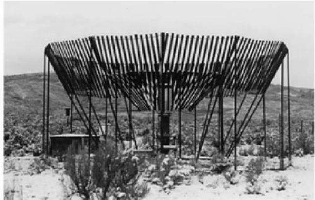
results (Table 4.4) show the necessity for the double fence installation, especially for solid precipitation. Moreover, at wind speeds  $> 5 \text{ m s}^{-1}$ , some correction for wind speed is required even for fenced gauges.
