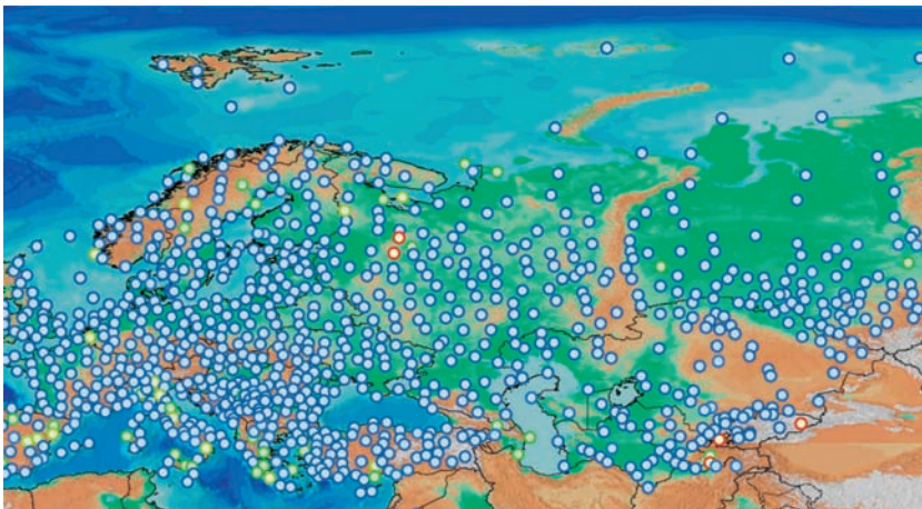
Figure 4.3. Map of the Weather Stations that Report Surface Weather to the World Meteorological Organization for Global Sharing and Analysis
