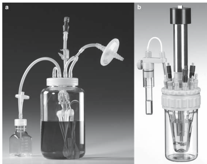
Fig. 5.3 Special bioreactors for small-scale and process development. (a) Superspinner, Membranreactor with tumbling membrane basket for bubble free aeration, Sartorius AG, Prof. Lehmann, University of Bielefeld (courtesy of Sartorius AG, Germany); (b) conical reactor (courtesy of medorex, Germany)
