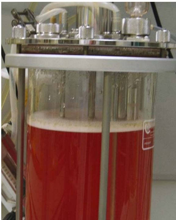
Fig. 4.27 5–10 mm foam layer at the medium surface (cell line: CHO-easyC – CHO-K1 derived line, Cell Culture Technologies GmbH, Zürich, Switzerland; CHO-master HP-1 medium; aerated with a ceramic micro sparger Fig. 4.18
