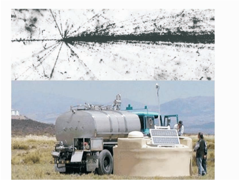
Figure 6.9: A collision between a high-energy cosmic ray particle and an atom in a photographic emulsion (viewed through a microscope). Below: filling of a water tank of the Auger observatory.
