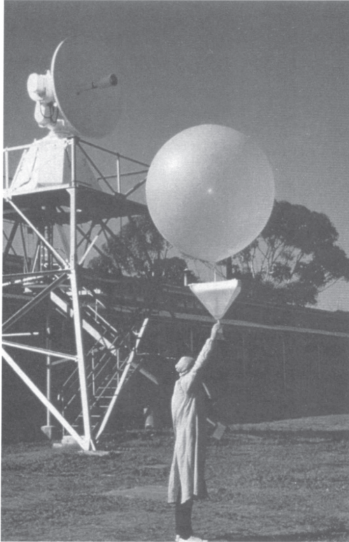
Plate 1.1 Releasing a balloon carrying a radiosonde to measure temperature and humidity conditions in the troposphere and lower stratosphere. The radiosonde equipment is in a box in the meteorologist's left hand. The box is attached by a cord to the pyramidal radar reflector which hangs beneath the balloon. The reflector enables location of the balloon's position by means of the radar equipment seen behind, and the change of position shows the sideways displacement (i.e. the wind) at each height. Notice that the meteorologist is wearing protective clothing in case the hydrogen in the balloon ignites, which is possible in dry conditions.
