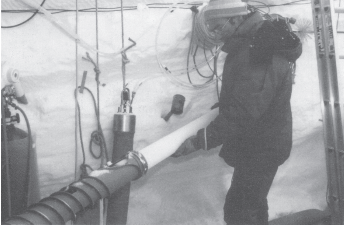
Plate 15.1 Evidence on past climates can be derived from the analysis of ice, and the bubbles of air within it, from various depths in Antarctica. The photograph shows a rod of ice being handled in an ice cave, after having been extracted by means of a vertical hollow drill mounted at the surface. The drill may be many hundreds of metres long, allowing the examination of ice of great age.
