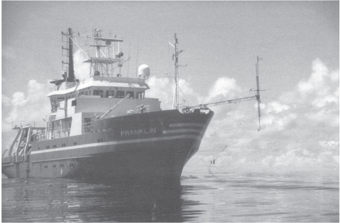
Plate 11.1 The oceanographic research vessel Franklin of the CSIRO Division of Oceanography, Hobart. This photograph was taken during experiments in the warm pool of the western Pacific, when a boom forward of the bows carried instruments for measuring the fluxes of heat and moisture from the water surface upwards, and of momentum downwards. The boom also carried an instrument to be lowered into the water for measuring the profiles of temperature and salinity within the upper 3 metres. Other instruments on the foremast repeated the flux measurements, and measured rainfall. Shortwave and longwave radiation were determined by instruments above the wheelhouse. Other instruments were towed from the afterdeck to determine the temperature and salinity profiled to 300 m depth.
