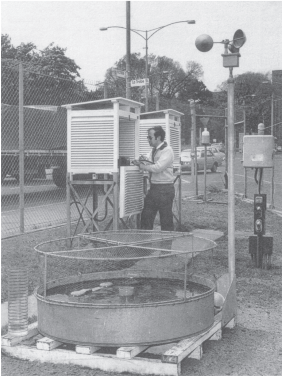
Plate 4.1 A US Class-A evaporation pan at a climate station in Melbourne. It is covered by mesh to exclude birds, whose drinking or splashing of the water would affect the daily lowering of water level due to evaporation. The congestion of the equipment and the undue proximity to a busy street are unfortunate but typical consequences of the growth of a city.
