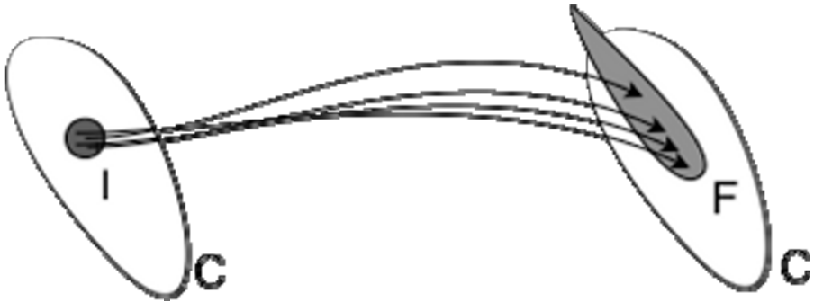
Figure 1. Schematic process of an ensemble prediction system. This is a procedure which maps a small subset of climatology, the analysis uncertainty (dark grey on left-hand side), into a generally larger subset of climatology, the forecast uncertainty (light grey on right-hand side). F may, in fact, include unphysical states.
