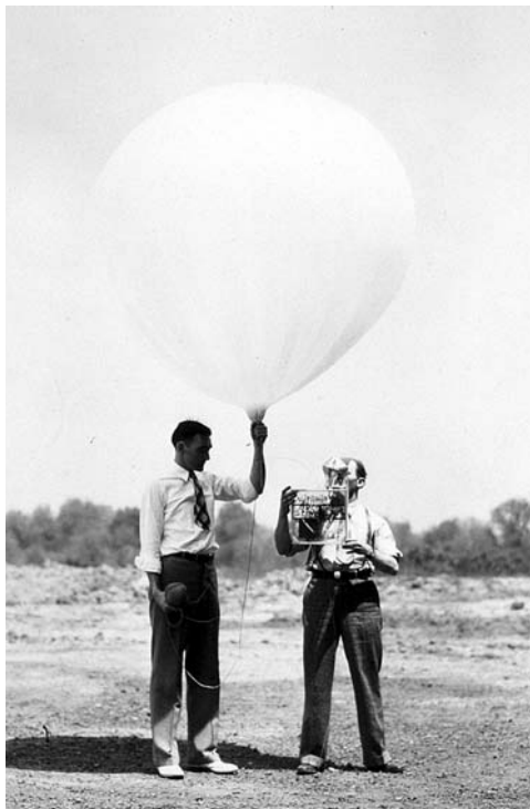
An early launch of a radiosonde by the U.S. Bureau of Standards. (NOAA)
