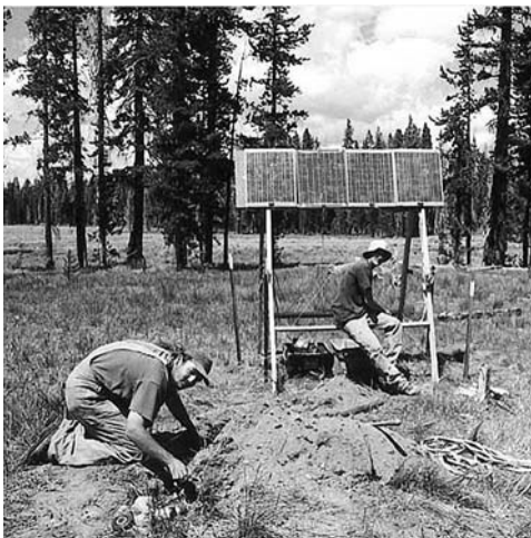
Expert geologists at Yellowstone's volcano observatory are constantly monitoring the region's underground activity. In this photo, a special seismic instrument is being installed. (Bob Smith/University of Utah/U.S. Geological Survey)
