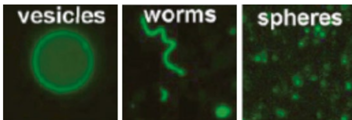
Fig. 8.4 Fluorescence microscopy images of OCL aggregates in water using the hydrophobic dye PKH26 (reprinted with permission from Rajagopal et al. (2010a). Copyright 2010 American Chemical Society)
