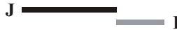
Fig. 2.8. A single pixel at the end of one segment might change the relationships significantly. We may have ( >(I,J)=1 and mi(I,J)=0 and oi(I,J)=0 ) or ( >(I,J)=0 and mi(I,J)=1 and oi(I,J)=0 ) or ( >(I,J)=0 and mi(I,J)=0 and oi(I,J)=1 ).
