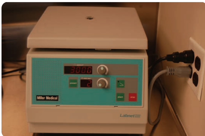
Figure 3-27: The centrifuge is shown with the desired settings of 3000 rpm at 2 to 3 minutes spin time. Generally, a spin cycle of anywhere between 2 to 3 minutes at a rate of between 2000 to 4000 rpm is acceptable.
