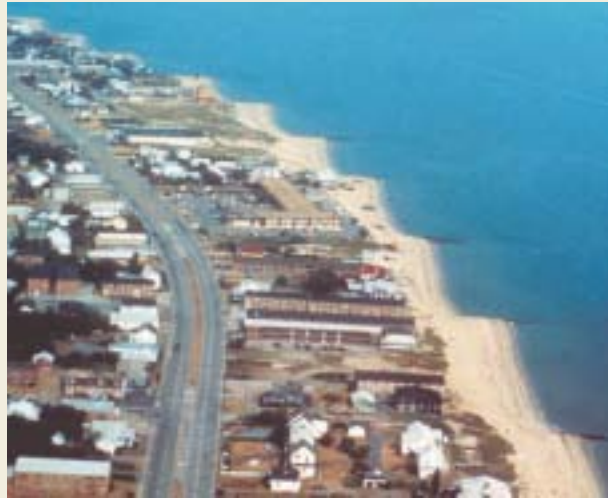
Groins on the Atlantic shoreline in Norfolk, Virginia, capture sand to maintain the beach.
