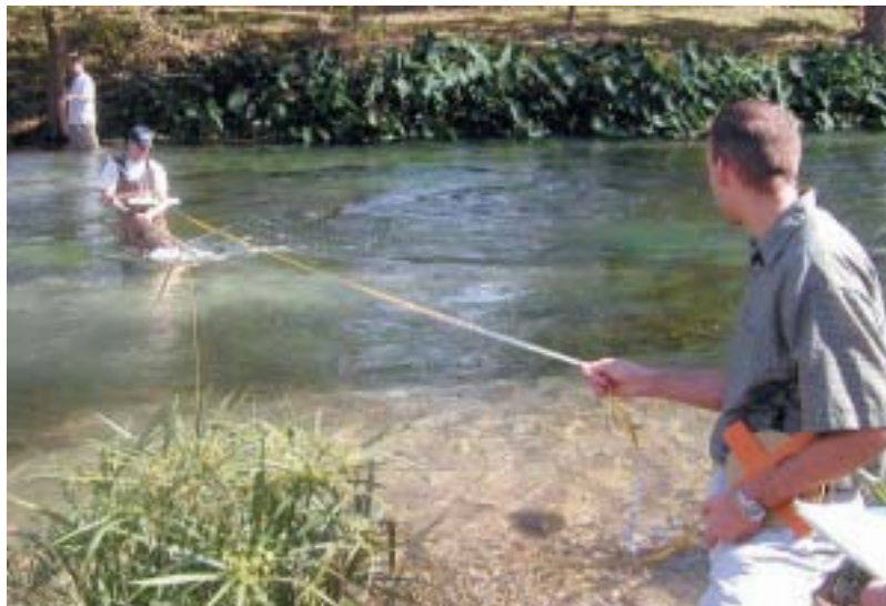
FIGURE 17.10 These university students are measuring a stream’s velocity, depth, and width in order to find discharge, the volume flowing in a stream per unit time.
