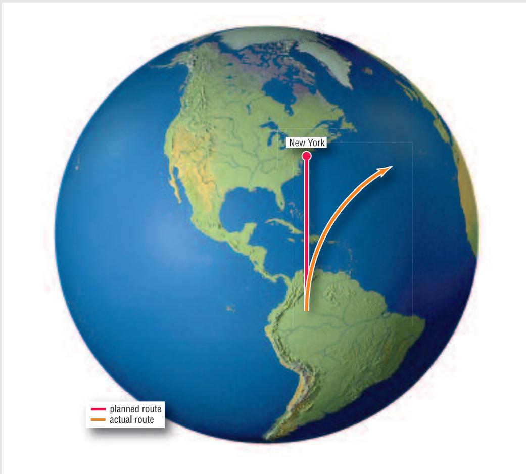
*Consequences of the Coriolis effect. An airplane heading for New York and flying due north will be deflected to the right on a path taking it out over the Atlantic.*
