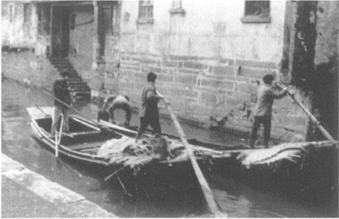
PLATE 16.6 Overloaded 'cement boats' carrying liquid sewage along a canal in Suzhou, Jiangsu Province, China. The boats themselves are made of cement but do not carry it, as the name might suggest
