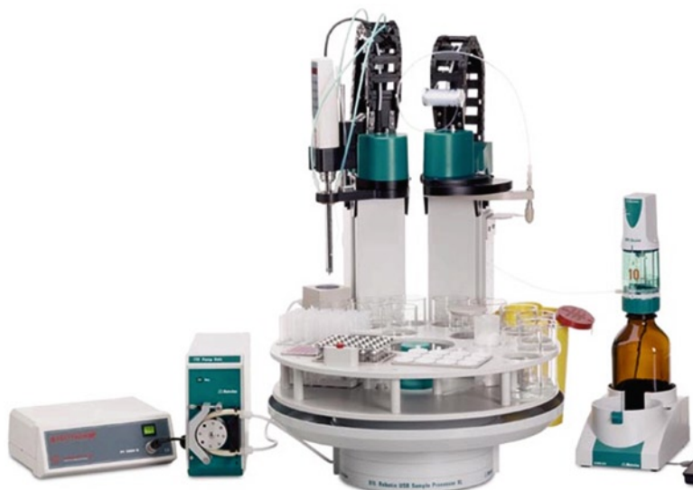
Fig. 12.10 Metrohm Robotic Soliprep system (reprinted with permission from Metrohm)
