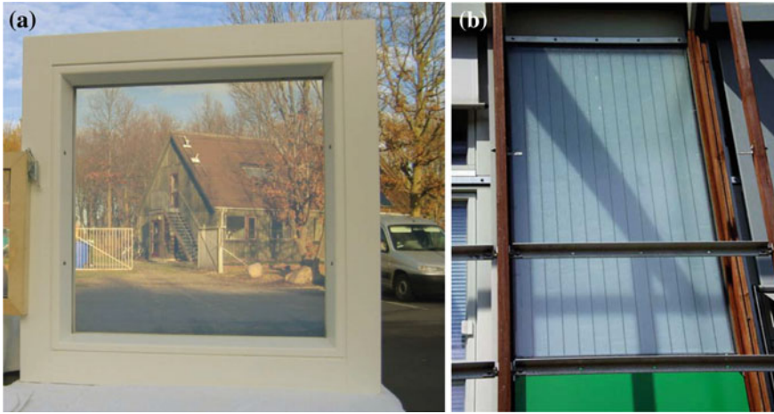
Fig. 3.2 Example of aerogel glazings: a evacuated prototype with monolithic aerogel (Schultz and Jensen 2008); b prototype of a PMMA system with granular aerogel installed on ZAE building in Würzburg (Reim et al. 2005)
