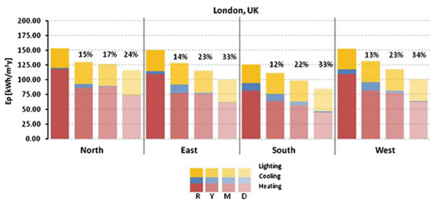
Fig. 6.11 Specific total primary energy use for different orientation and reaction time of the ideal adaptive glazing material for the climate of London ( R = Reference, Y = Yearly optimised, M = Monthly adaptiveness, D = Daily adaptiveness.). Percentages indicate the energy savings compared to the R static glazing material. As published by Favoino et al. (2015a), under CC-BY licence
