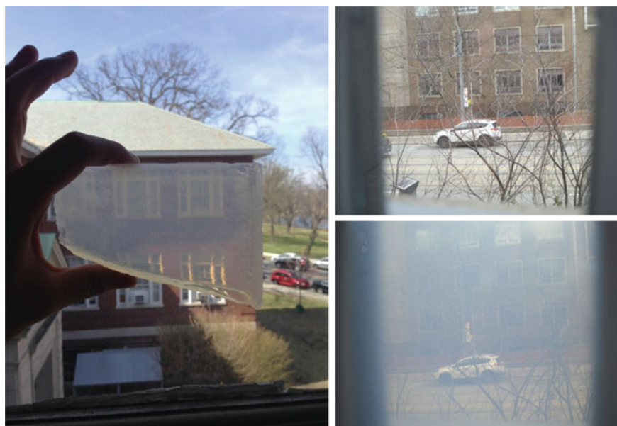
Fig. 3.5 Aerogel effect on the vision by comparing the double glazed unit with and without the monolithic aerogel panel (Berardi 2015)
