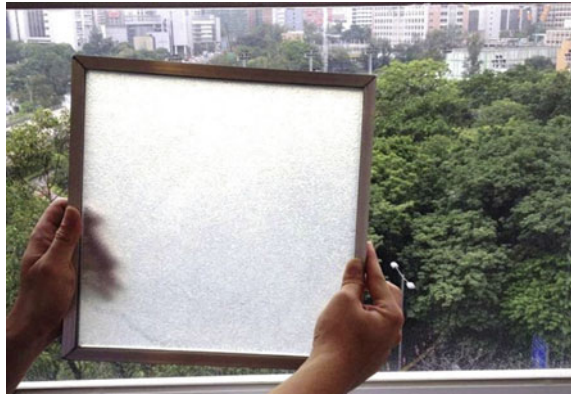
Fig. 3.6 Effect of granular aerogel on the vision through a window (Huang and Niu 2015a)
