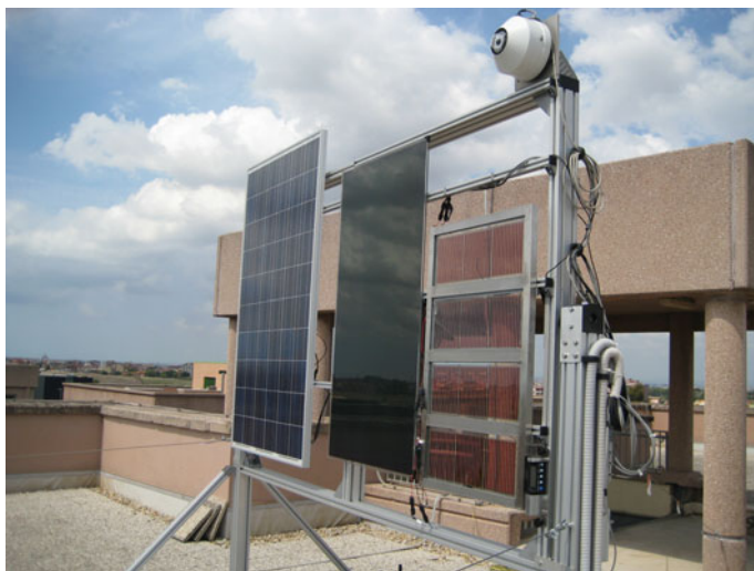
Fig. 11.10 Vertical configuration test bed for comparative analysis of DSM with other technologies
