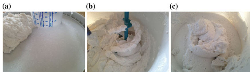
Fig. 2.5 Various steps of the mixing: (a) original components; (b) mixing phase; (c) final composition of the plaster (Buratti et al. 2014)
