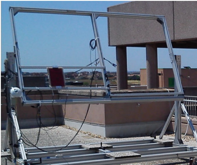
Fig. 11.7 Experimental set-up for AOI measurements at ESTER laboratory
