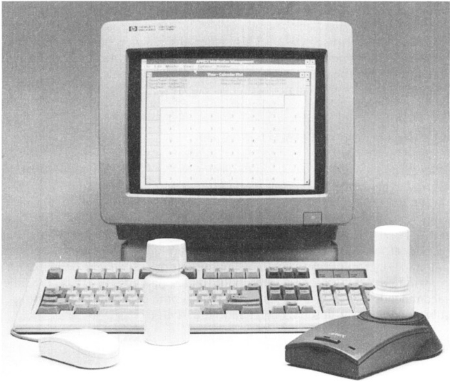
FIG. 1. Electronic medication event monitor in the process of communicating stored data from monitor to computer. The transfer occurs without wire connection between the inverted monitor and the communications interface device, which transfers data to MS-DOS-based computers via serial port. A second medication event monitor, with a somewhat larger container size, stands nearby. (Copyright, 1994, APREX Corporation; reproduced with permission.)
