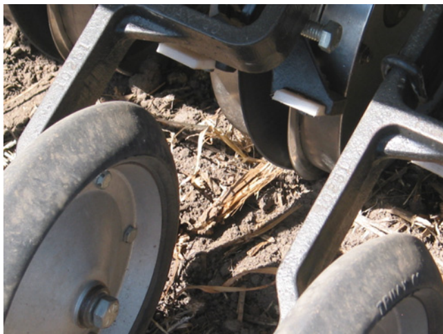
Figure 5.1 Depth bands on grassland drills regulate the depth with which small-seeded perennial grass seeds are placed below the soil surface. Switchgrass should be seeded no deeper than 1.25 cm below the soil surface to promote rapid establishment.
