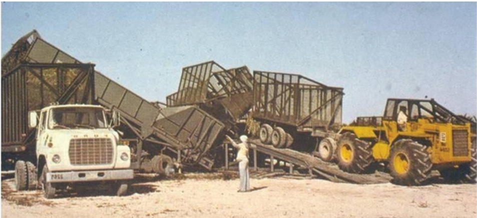
Figure 13.6 Transfer of sugarcane from in-field hauling trailers to highway-hauling trucks. (Photo credit J. Cundiff © 2013).
