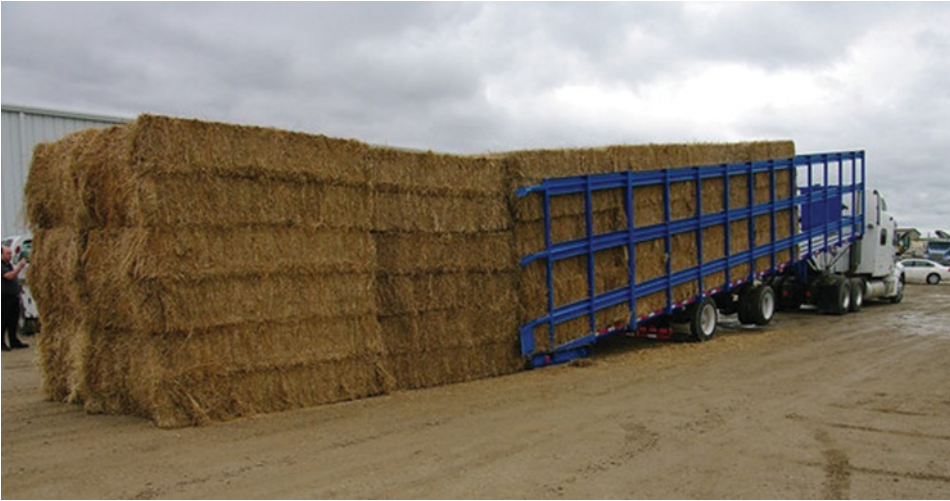
Figure 13.10 Self-loading trailer built by Kelderman Mfg. to implement multibale handling unit concept for 36-bale stack of 3 \times 4 \times 8 ft rectangular bales. (Image courtesy of Kelderman Mfg. Reprinted with permission, K. Comer, personal communication).
