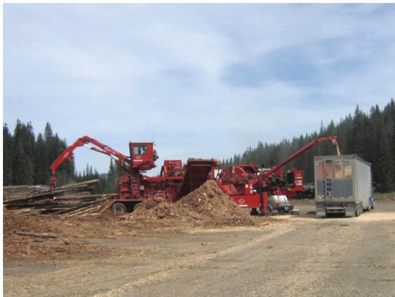
Figure 14.7 A complete mobile chipping unit processing de-limbed small-diameter logs from a commercial thinning operation into clean chips in north Idaho. The chipping is located at a concentration yard 2–3 miles from where the trees were harvested. (Photo: © Keefe, 2013).
