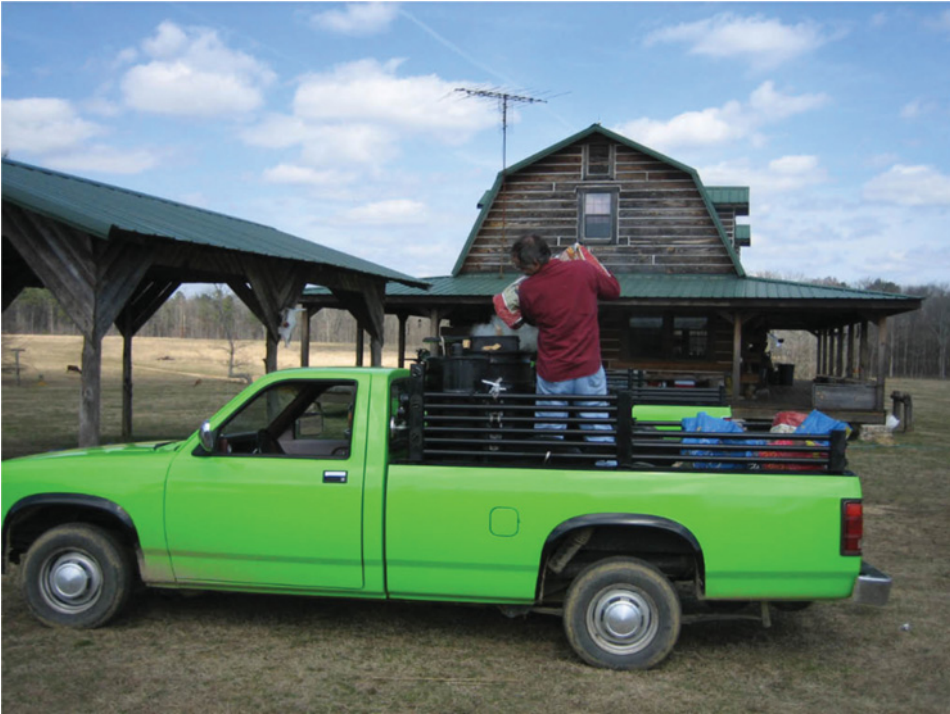
Figure 10.4 In countries where gasoline was in short supply during the Second World War, people converted their vehicles to run on wood gas (also known as producer gas). Dr. South currently owns a 1989 truck that was modified to run on either gasoline or wood. This truck travels about 8.5 km using either a liter (0.72 kg) of gasoline or 2.4 kg of dry pine blocks ( \approx 14\% od moisture content) (© 2013, South).
