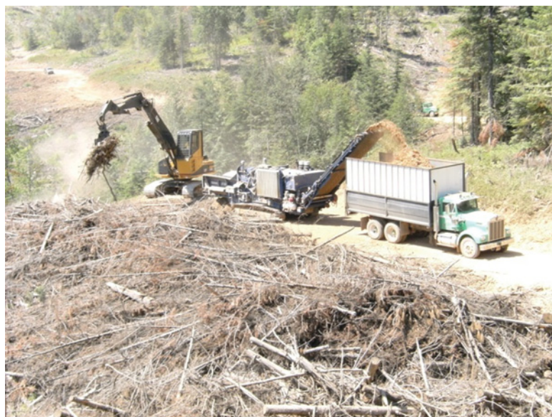
Figure 14.8 A loader feeds a horizontal grinder, which in turn fills a high walled dump truck being used to haul biomass over a low volume forest road to a concentration yard. (Photo: © Anderson, 2013).
