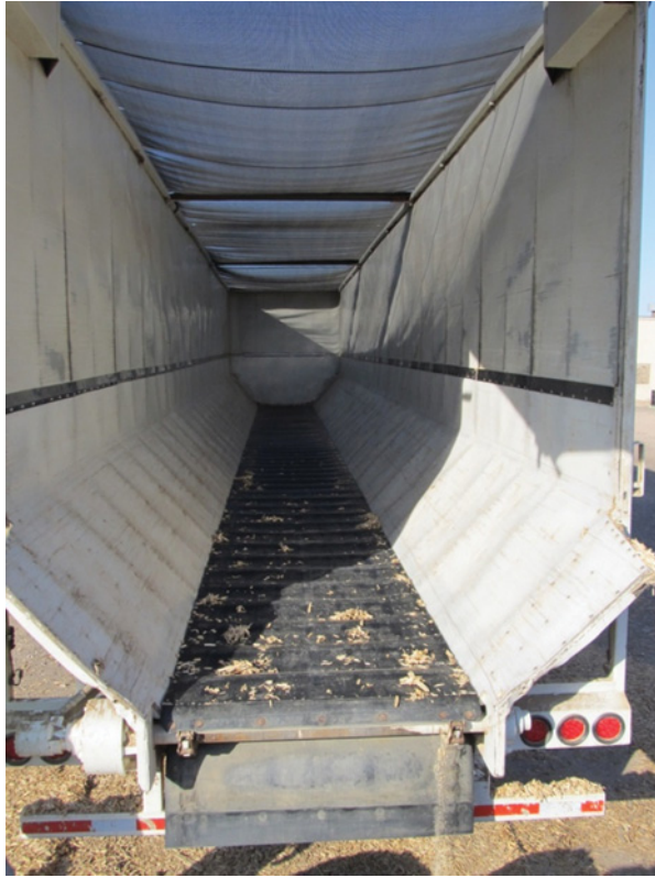
Figure 14.9 The back of a walking floor trailer that allows for automatic unloading of comminuted biomass. (Photo: © Anderson, 2013).
