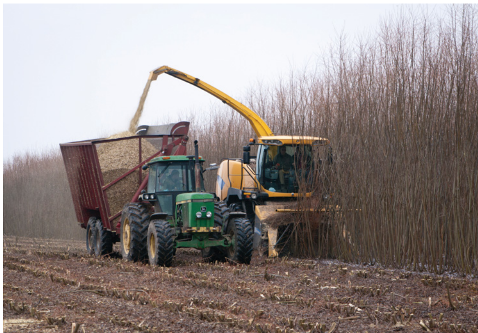
Figure 12.4 Harvesting four-year-old willow biomass crops with a cut and chip harvesting system based on a New Holland FR self-propelled forage harvester and a New Holland FB 130 coppice header that was designed for woody crops like willow and hybrid poplar (Photo credit D. Angel © SUNY ESF).
