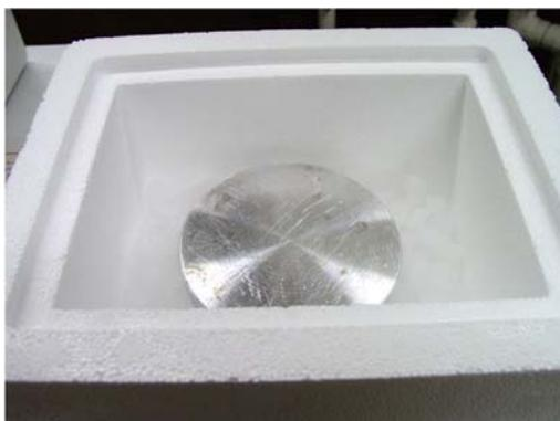
**Fig. 3** Aluminum disc, approximately 125 mm in diameter  $\times$  15 mm, on dry ice inside a Styrofoam shipping carton.
