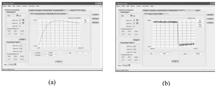
Fig. 3 – Graphical user interfaces (GUI) of the Web application. (a) On-line remote monitoring of the Phe released during hydrolysis with CPA. (b) Remote pH control of WPC production: servo problem.
