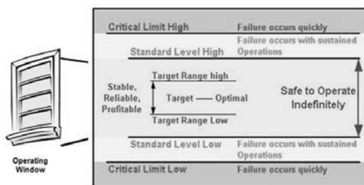
Fig. 2 Concept of IOW system (“Establishing Integrity Operating Windows (IOW’s)”, John Reynolds)
