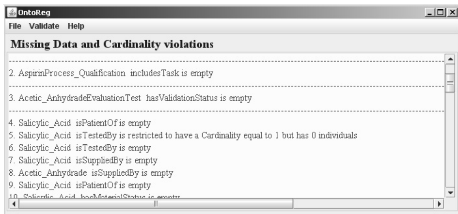
Figure 3. The Missing Data warning: a supplier has to be assigned for Salicylic_Acid.
