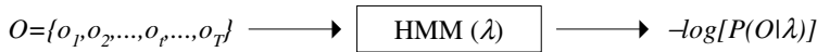
Fig. 1. Input-output relation for HMMs: observation sequence (O) and likelihood value ( -\log[P(O|\lambda)] ), respectively.
