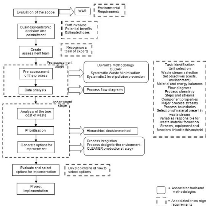
Figure-1 Main strategy for waste minimisation with associated knowledge requirements methodologies and tools
