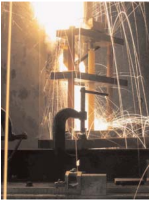
Picture of a floating roof to shell shunt test (submitted to a 830 A current to simulate lightning) showing the sparks generation (note that wax and rust deposits increase sparking).
