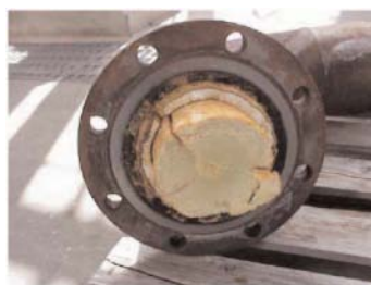
(Left) Polymer plugging the polymer catch tank vent nozzle. (Right) Vent line obstructed by solid polymer.
