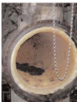
Polymer catch tank after the incident. Its cover was blown a few feet away.
