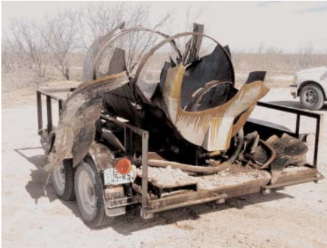
The ruptured blowdown tank.
