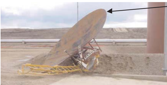
The tank roof and its associated structure on the ground.
