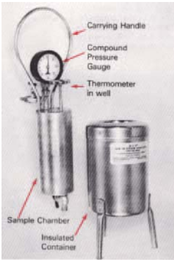
Figure 5a MSA air-in-steam analyser. A simple, rugged instrument for measuring the quantity of noncondensables in steam was developed by the American Oil Company MSA. It works on the principle that the pressure of a steam-noncondensable mixture at a certain temperature indicates the percentage of noncondensables present.
