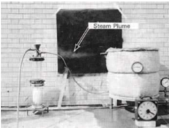
Figure 8a A mixture of steam and air is being fed into the drum. There is a show of steam at the vent. The thermometer in the vessel reads 140°F (60°C), indicating the vessel contains only 20 percent by volume steam.
