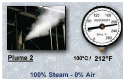
Figure 4 The gas coming out of the pipe nipple is pure steam. The dial thermometer indicates that the steam is at 212°F (100°C). The temperature outside was 60°F (15.5°C) when the picture was taken.
