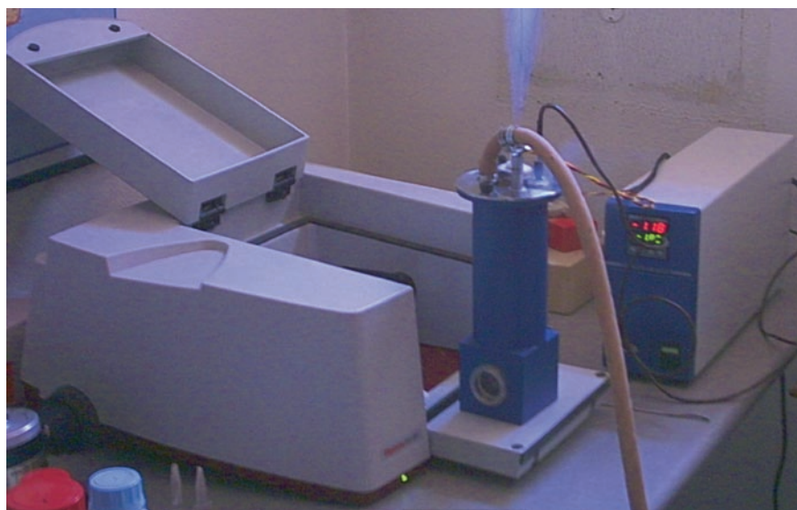
Fig. 10.1 The variable temperature cell ready to be installed inside the FT-IR spectrometer. Behind the cell, on the right, there is the temperature control unit
