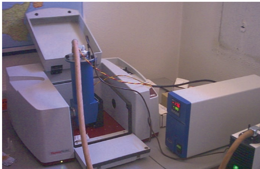
Fig. 10.2 The variable temperature cell installed inside the FT-IR spectrometer. The temperature control reports -176^{\circ}\text{C} (97 K)
