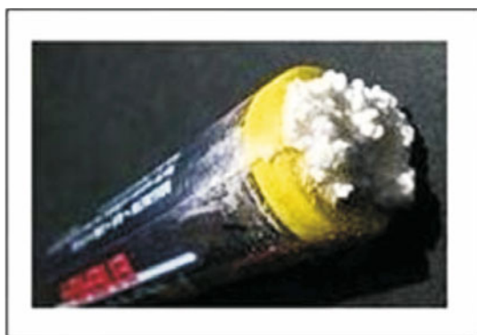
Fig. 14.3: Leaked alkaline battery.
