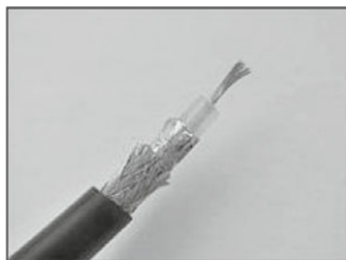
Fig. 15.2: Coaxial cable with dielectric insulator.
