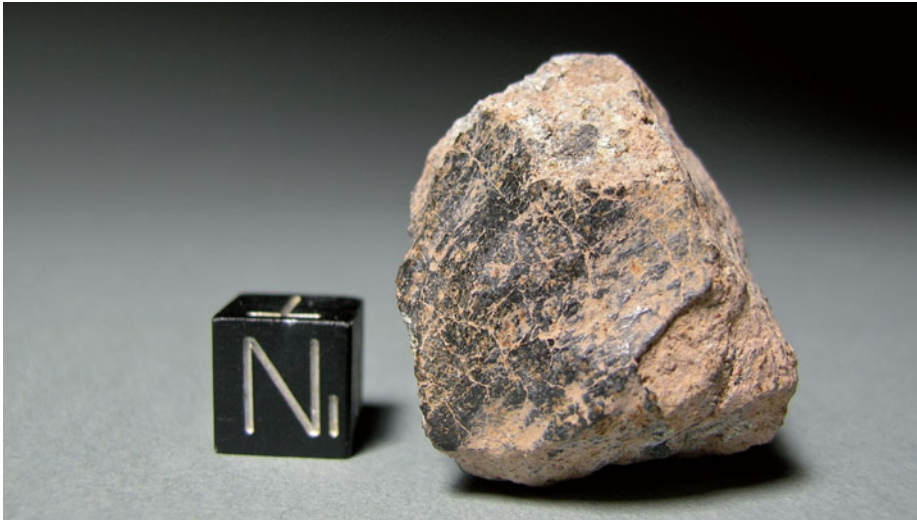
Carancas, 27.20 g fragment (Buhl Meteorite Collection # B-203). The Carancas meteorite fell at 16:40 UTC on September 15, 2007 in Chucuito province, Peru. The impact of the mass, which had not fragmented prior to impact, formed a crater 4.5 m deep and 13 m in diameter. Carancas is a H4–5 ordinary chondrite. The surface pictured shows a black shock plane. Photo: S. Buhl
