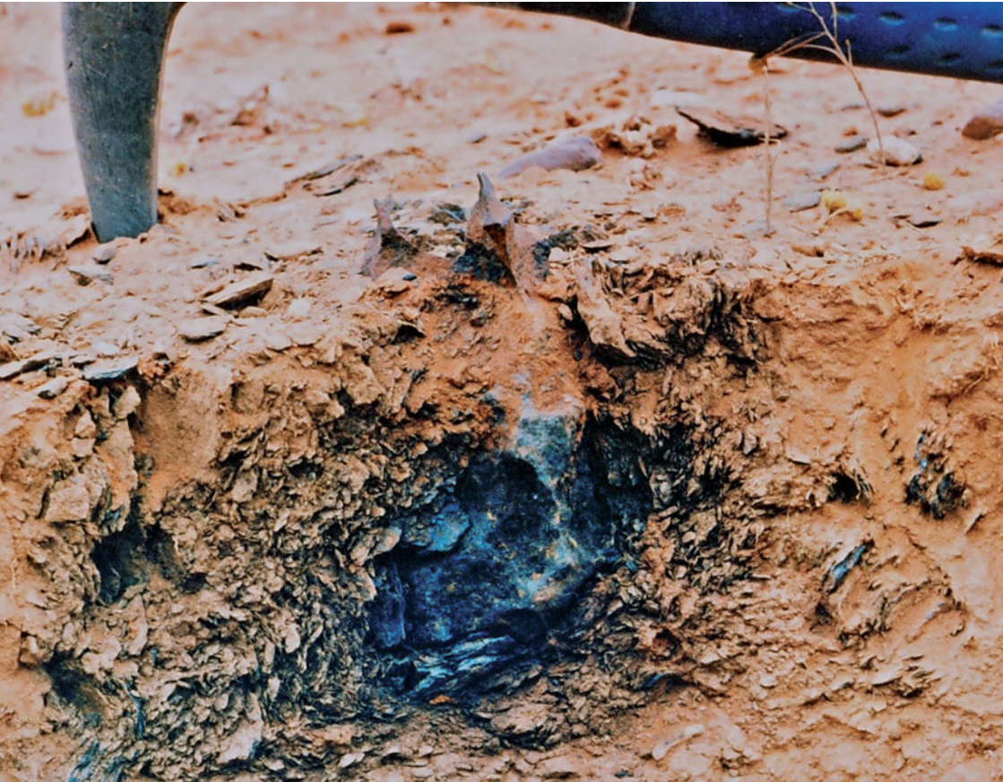
Henbury meteorite in situ. The 950 g specimen is embedded in the top soil to a depth of 10 cm and surrounded by a relatively thin aureole of rust. Caliche has coated the portion of the meteorite near the surface. Note the characteristic spikes protruding from the top soil which indicate a strong degree of ablative weathering. Geologist hammer for scale comparison. Photo: D. McColl
