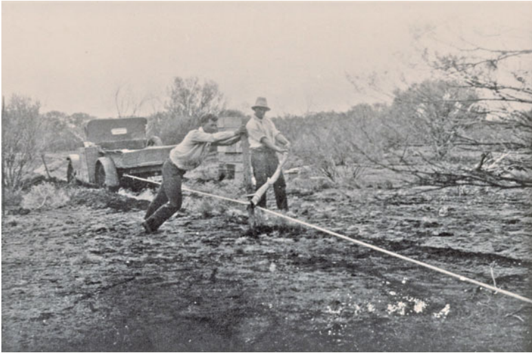
“Bogged. Bill Bedford & Ben Peters. Truck unloaded and being pulled out with Spanish windlass .” Photo taken on the way from Henbury to Coober Pedy, August 1931. Bedford Papers, Barr Smith Library, University of Adelaide, MSS 92 B4113p
