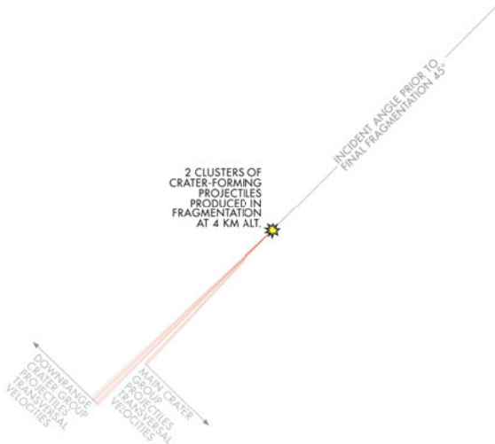
Schematic W - E lateral view of the final catastrophic disruption that produced the two crater-forming projectile clusters. The specific transversal velocities and resulting incident angles of the respective projectiles are controlled by the position of the trajectory's terminal point, which in turn is defined by the projectile masses. In order to reproduce the existing crater distribution pattern, the fragmentation-induced velocities transverse to the flight path were adjusted, and the resulting order of magnitude for the transversal velocities in this scenario is 200 m/s on average. The values for the masses producing the large craters are lower, those for small craters and big individuals are higher by a factor of around 2 in both directions, reflecting the momentum transfer by the fragmentation mechanism. Due to hypervelocity conditions ballistic curvature is not relevant at this scale. Numeric modeling by K. Wimmer, diagram S. Buhl
