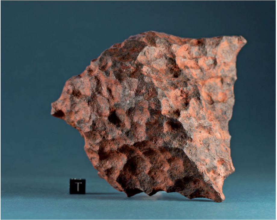
On describing Henbury meteorites Robert Bedford (1934) was the first to note that the size of the regmaglypts correlates with the dimensions of the respective meteorite. Krinov (1963, 1974), based on his study of meteorites from the Sikhote-Alin fall, later gave the ratio of the size of the regmaglypts to the size (cross section) of the meteorite as K = 0.09 . Pictured on the opposite page is a Sikhote-Alin individual of 3,600 g (cross section 162 mm) with an average regmaglypt diameter of \sim 14 mm. Pictured above is a 2,765 g Henbury individual (cross section 145 mm) with an average regmaglypt diameter of \sim 12 mm (max. dimensions measured). Scale cube is 1 cm. Photos: S. Buhl
