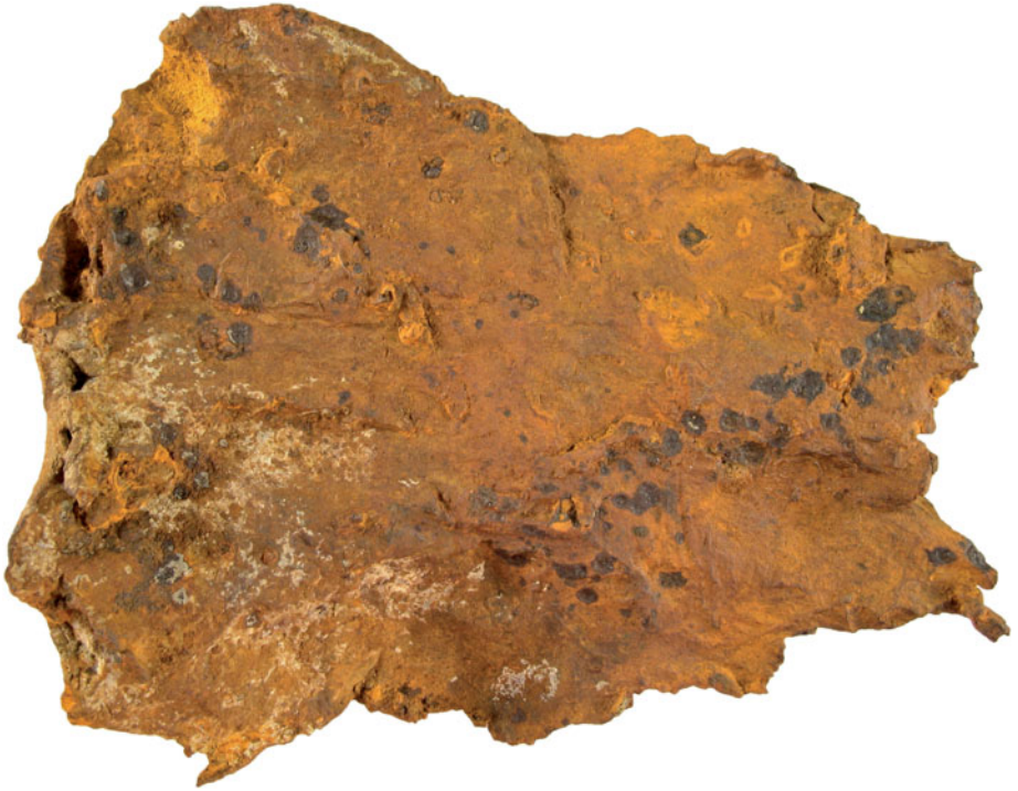
“Sample 9” in as found condition. It is the largest shrapnel recovered at Whitecourt. The exceptionally well-preserved meteorite measures 12.5 cm across and weighs 1,196 g. Photo: Chris Herd, Earth and Atmospheric Sciences, University of Alberta
