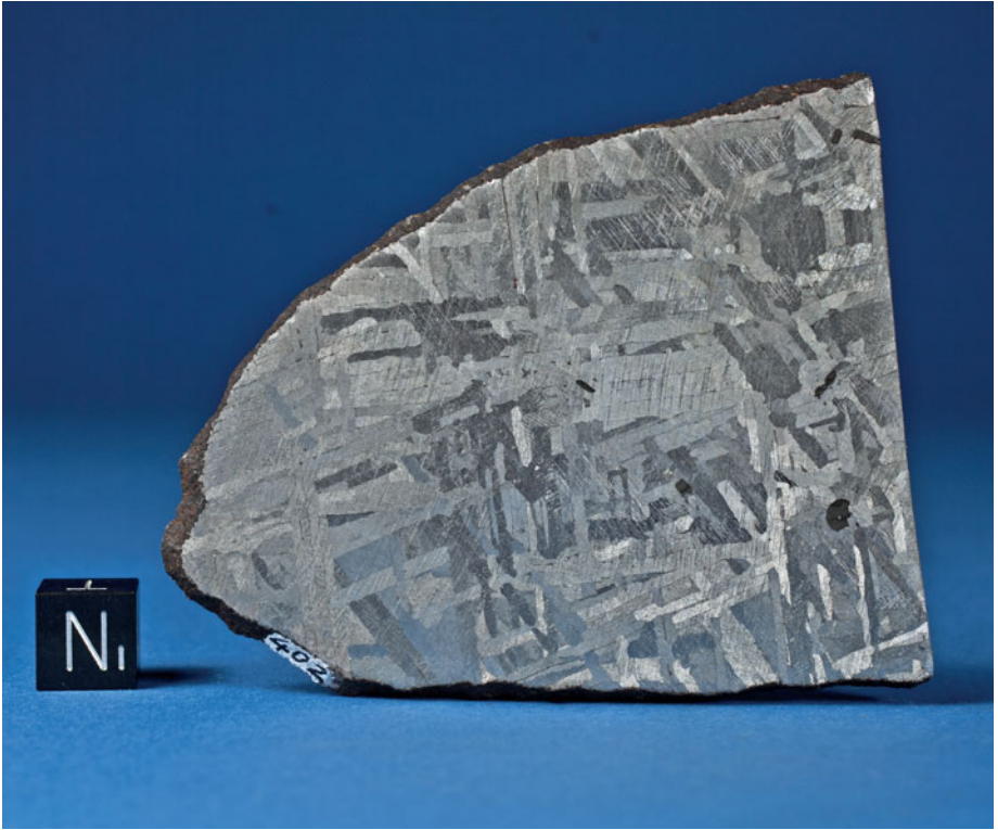
Top: Polished and etched cut section of a Henbury meteorite showing several small troilite nodules. The section taken from a flight ablated individual shows an undisturbed Widmannstätten pattern. Scale cube is 1 cm. Photo: S. Buhl. Left page: Henbury specimen of 45 kg exhibiting distinct atmospheric sculpting. This meteorite was donated to the Strehlow Centre Museum in Alice Springs where it is on display. Photo: D. McColl
