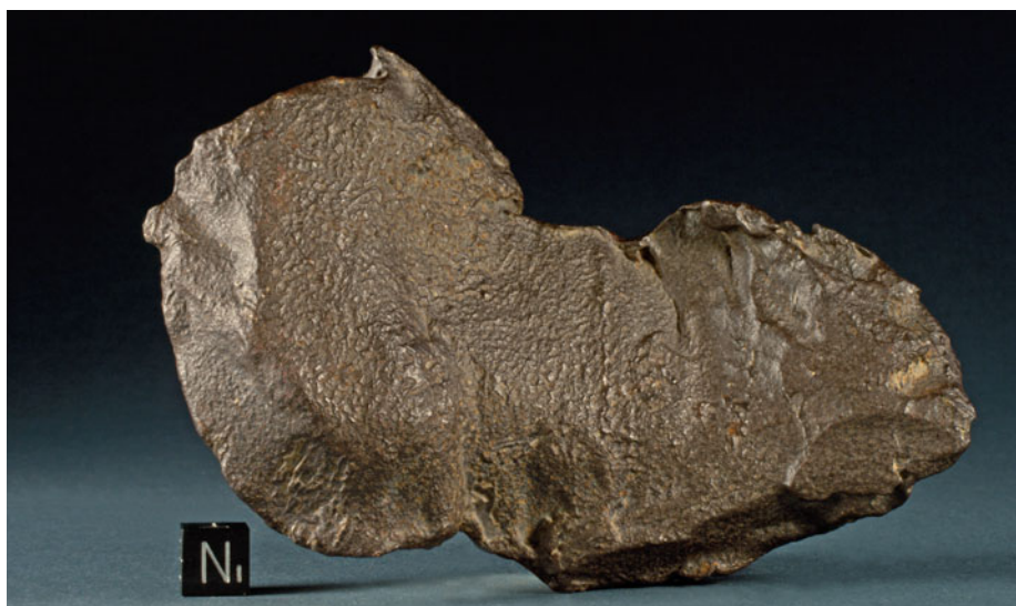
Opposite surface of the 739 g Gebel Kamil shrapnel. On its upper surface the specimen shows the typical weathering-pattern of iron meteorites exposed to corrosion (mechanical erosion) in hyper-arid climates and extreme temperature fluctuations. Photo: S. Buhl
